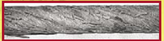
Figure 2: The untrimmed wires in this mining rope caused premature rope retirement.
