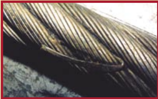
Figure 4: Damage from untrimmed broken wires was the cause of retirement in this rope.
