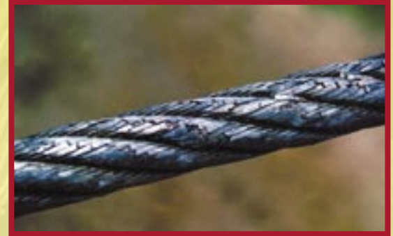
Figure 3: Worn drag rope with multiple crown and valley breaks.
