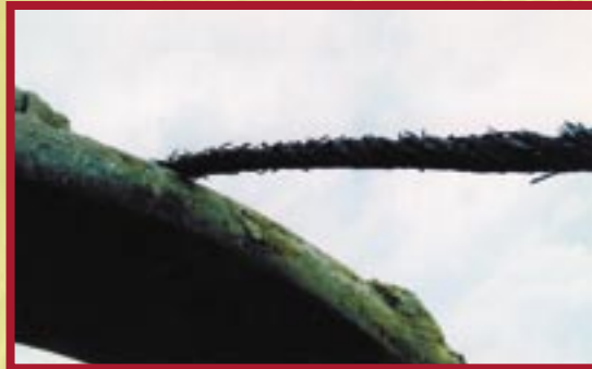
Figure 1: This dump rope shows severe abrasion.
