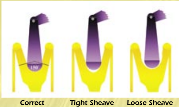
Figure 3: Cross sections illustrating three sheave groove conditions
