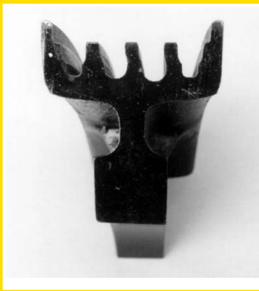
Figure 5 This sheave shows a number of defects that need to be corrected through either regrooving or sheave replacement: (a) the sheave alignment, of either this sheave or a secondary, needs to be assessed as the three of the four grooves (left to right) indicate ropes pulling to one side, as shown by the wearing of the groove. Unusual wear patterns and wire breaks along the wear plane will lead to premature rope retirement; (b) as a result of the improper sheave alignment, the first groove has developed a sharp edge on its right side where the rope has worn the groove; (c) likewise, the second groove also has a sharp edge, both of which will quickly abrade the rope; (d) differential groove depths, a result of improper tensioning, will further compromise the rope's service life.
