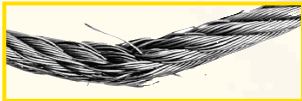
Figure 4: This 6-strand rope, showing extreme fatigue, operated in a reverse bend configuration. Note the number of crown and valley breaks.
