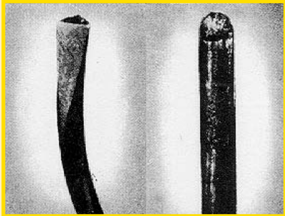
Figure 8: Both photos illustrate fatigue breaks. The fatigue break on the left is caused by abrasion, and is normally found on crown wires. To the right is a true fatigue break typically found to be the cause of valley breaks.
