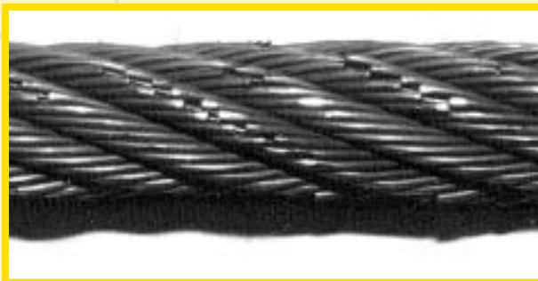
Figure 1: Crown Fatigue Breaks
